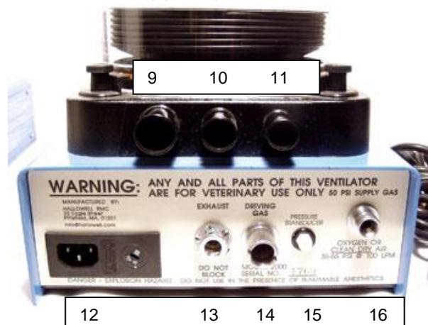
\* The following items should remain set up at all times: The blue exhaust hose connected to the breathing system exhaust port (10), the clear breathing system hose connected to the breathing system port (9), clear small tubing connected to the pressure transducer port, and to the circle system pressure adaptor, the driving gas control (14) and bellows (11) ports connected by black rubber hose.
