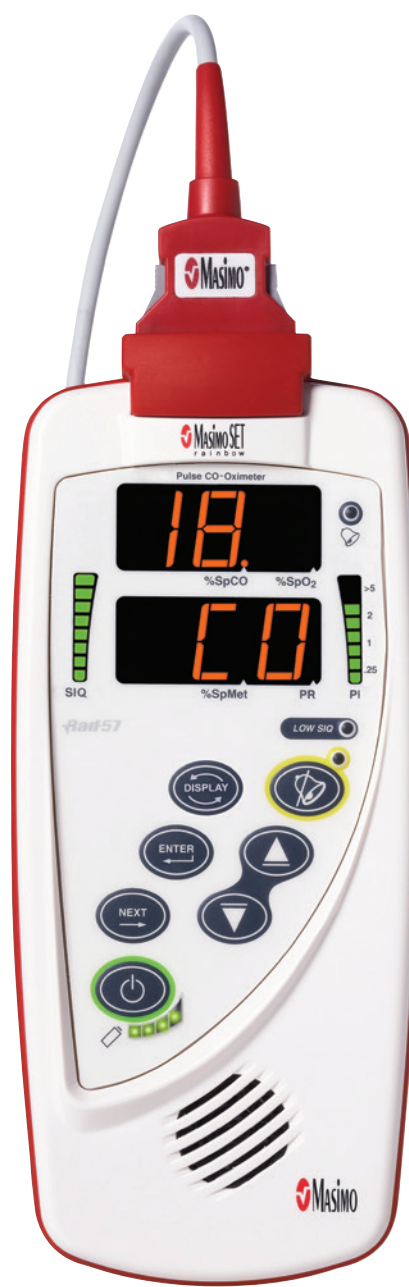
Pictured is the Rad-57 displaying SpCO. Display features will vary based on the noninvasive measurements loaded onto the device.
